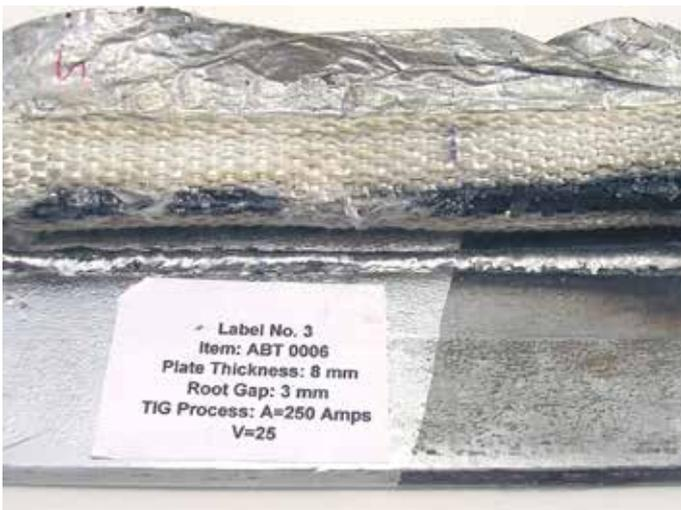
Weld bead achieved with Heavy Duty tape. 8 mm Plate with a 3 mm root gap at: 250 Amps.
