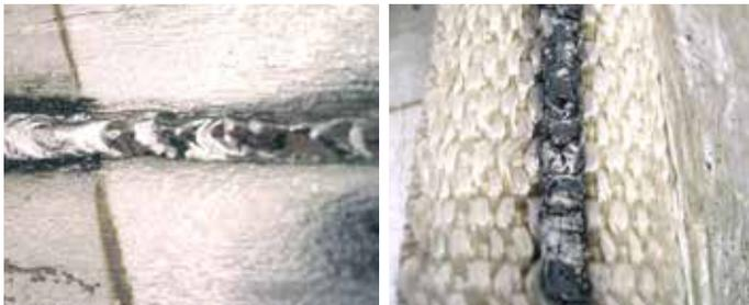
Light Duty tape used on 8 mm plate with a 3 mm root gap and a manual GTAW technique at 90 Amps.
